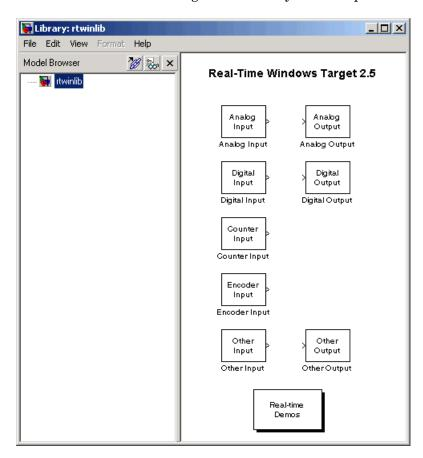
**2** Click and drag the Analog Input block to your Simulink model. Remove the Signal Generator block and connect the Analog Input block to the Transfer Function block.
