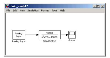
You next task is to enter parameters for the Analog Input block. See "Analog Input Block" on page 4-10.
